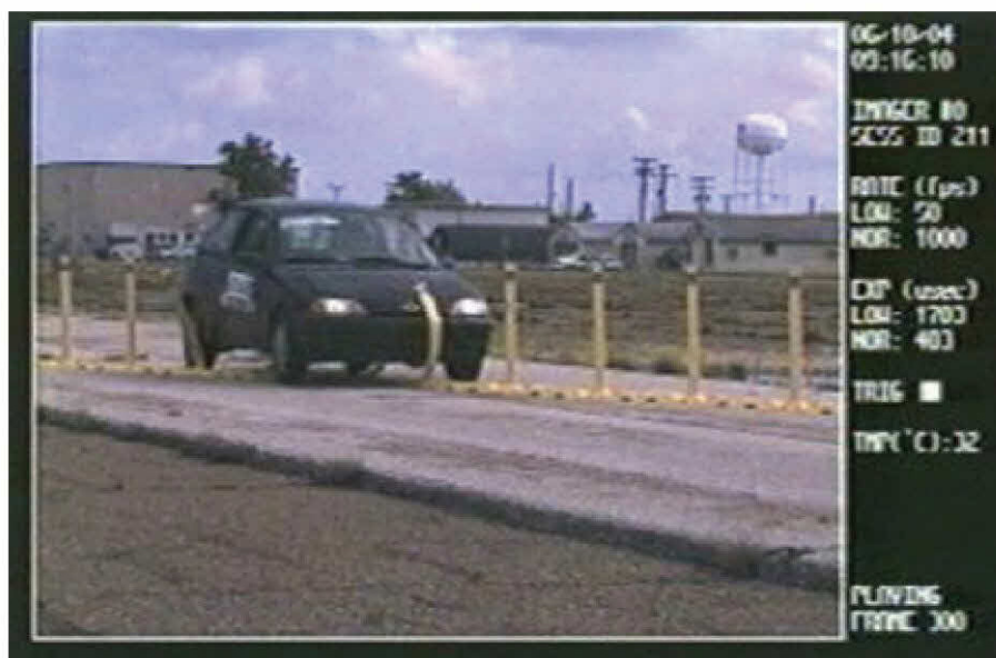
Texas Transportation Institute FG 300 Curb & Post 70 MPH Impact Test
